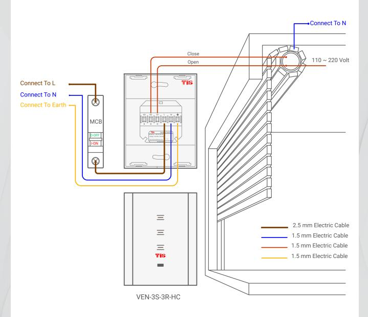
Figure 2: VEN-3S-3R-HC Motors Connection Diagram
