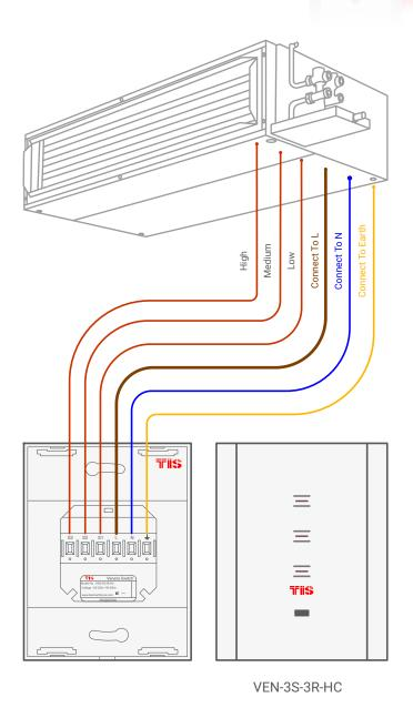
2.5 mm Electric Cable 1.5 mm Electric Cable 1.5 mm Electric Cable 1.5 mm Electric Cable
