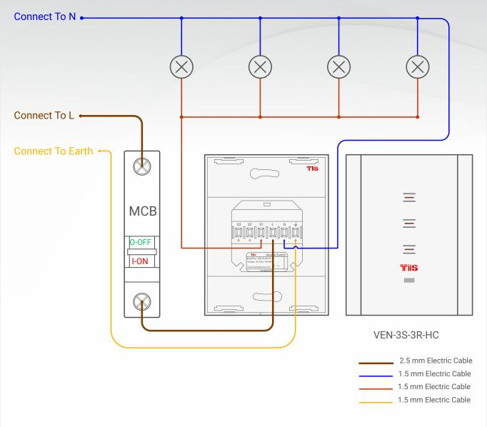
Figure 1: VEN-3S-3R-HC Lights Connection Diagram
