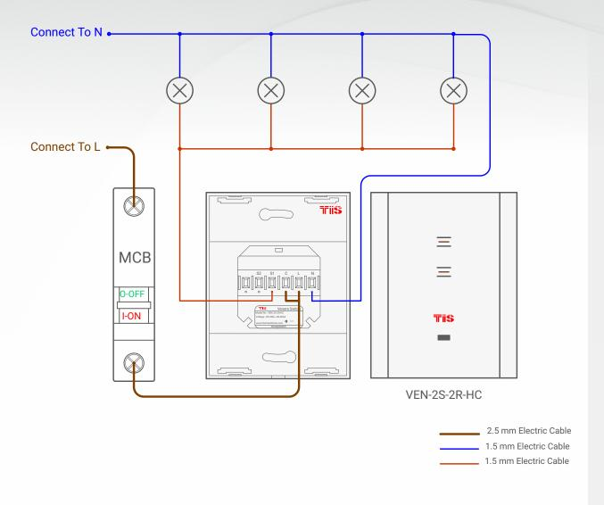
Figure 1: VEN-2S-2R-HC Lights Connection Diagram
