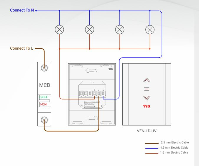
Figure 1: VEN-1D-UV Lights Connection Diagram
