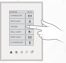
3>> Test by pressing the wall panel's ON/OFF button. The AIR Plug relay should respond by turning ON and OFF accordingly.
