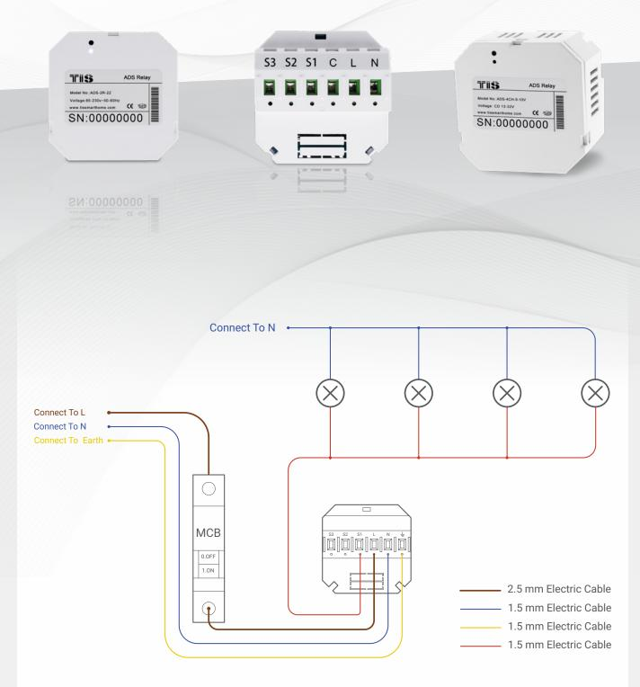
Figure 1: Lights Connection Diagram
