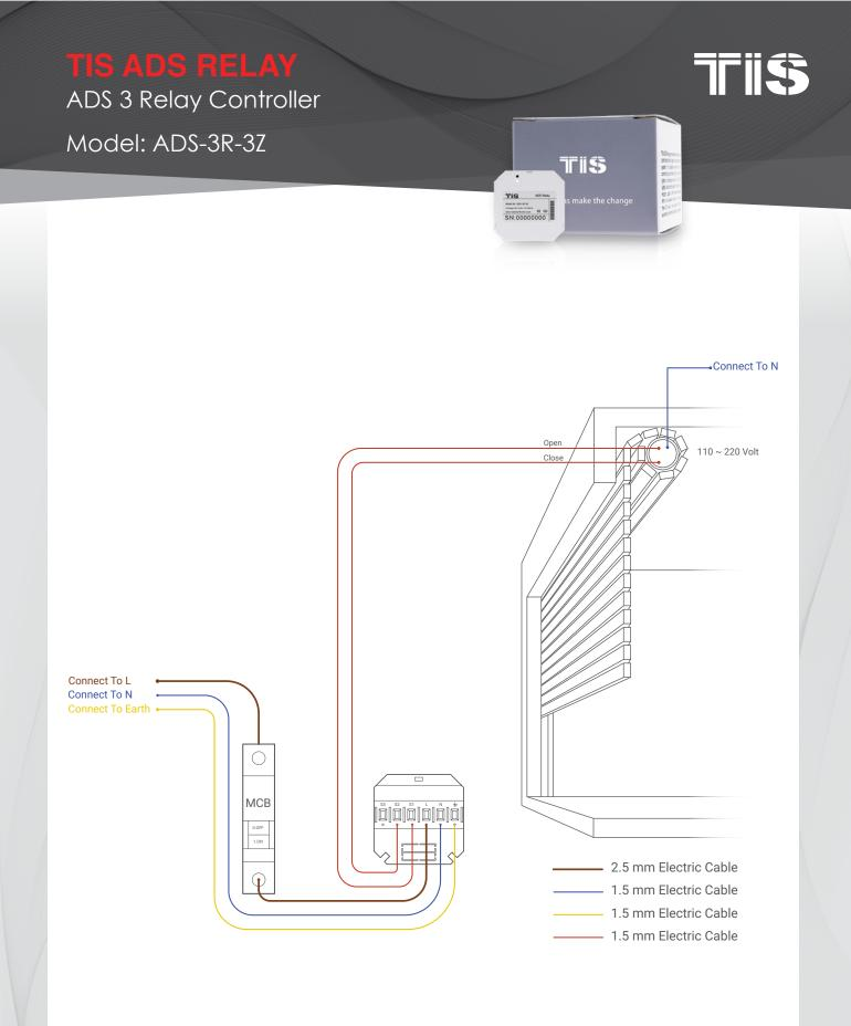
Figure 2: Motors Connection Diagram
