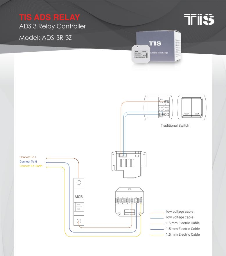
Figure 7: Traditional Switch Connection Diagram
