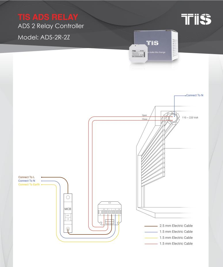
Figure 2: Motors Connection Diagram
