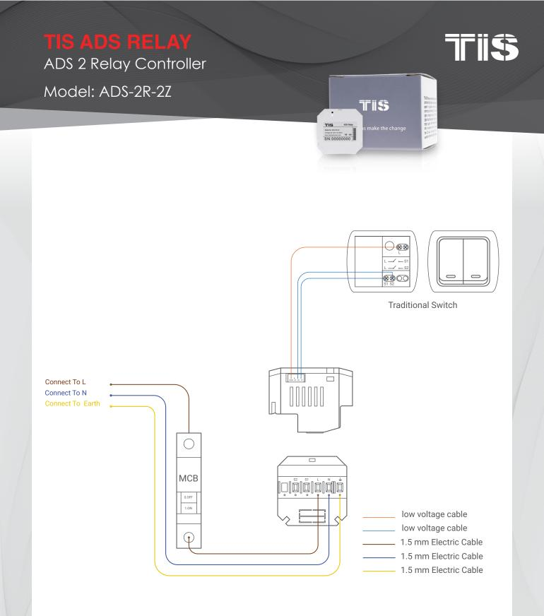
Figure 5: Traditional Switch Connection Diagram
