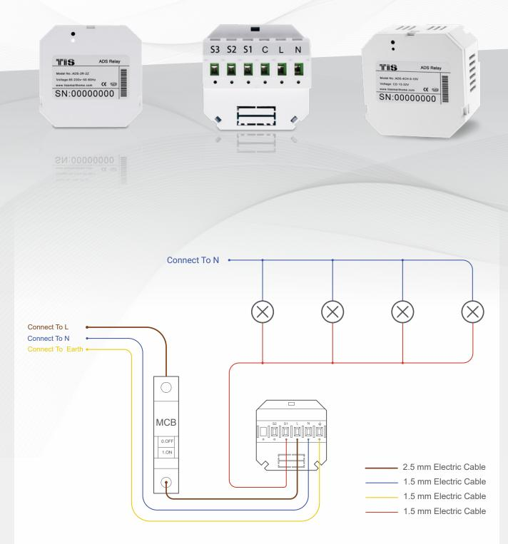
Figure 1: Lights Connection Diagram
