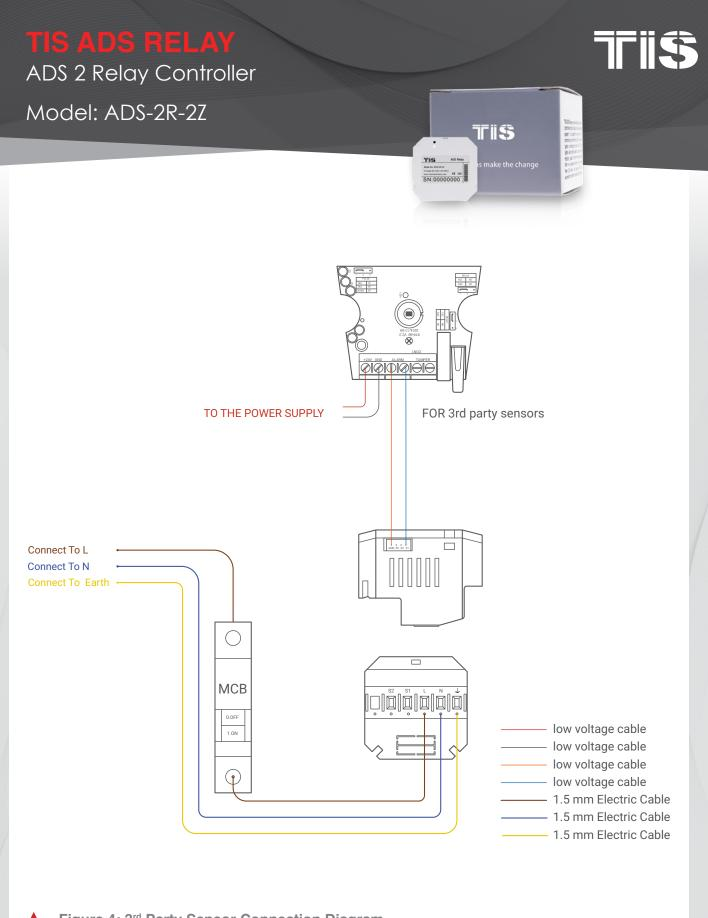
Figure 4: 3<sup>rd</sup> Party Sensor Connection Diagram
