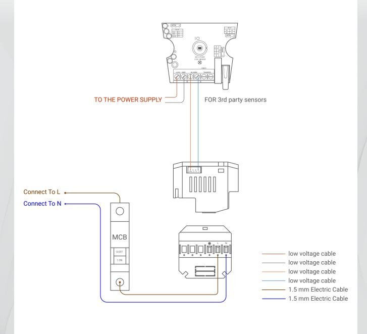
Figure 3: 3<sup>rd</sup> Party Sensor Connection Diagram
