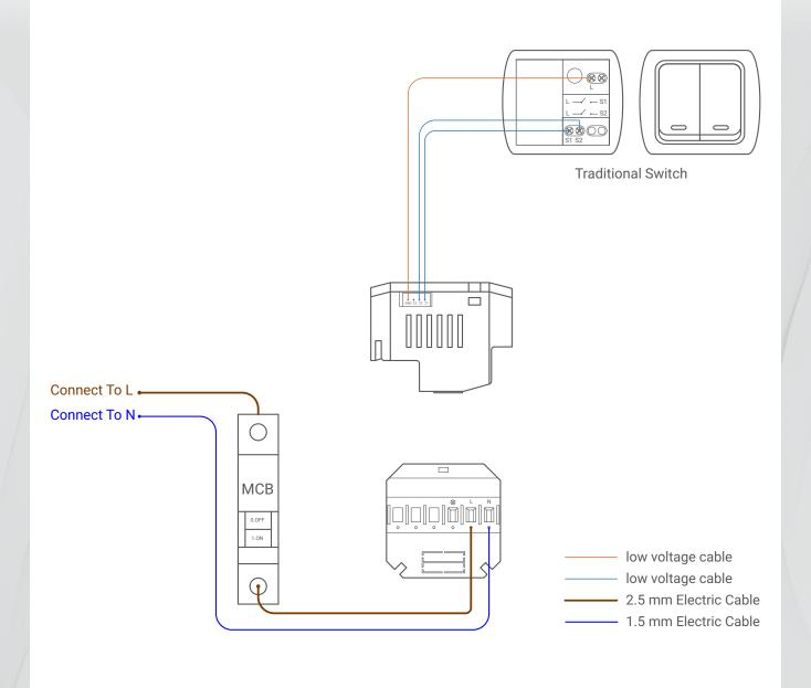
**Figure 4: Traditional Switch Connection Diagram**
