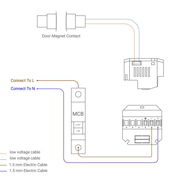
**Figure 2: Magnetic Door Contact Connection Diagram**
