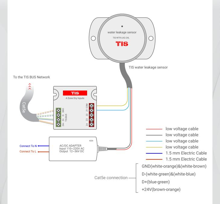
Figure 1: 4-Zone Dry Input & TIS Water Leakage Sensor Connection Diagram
