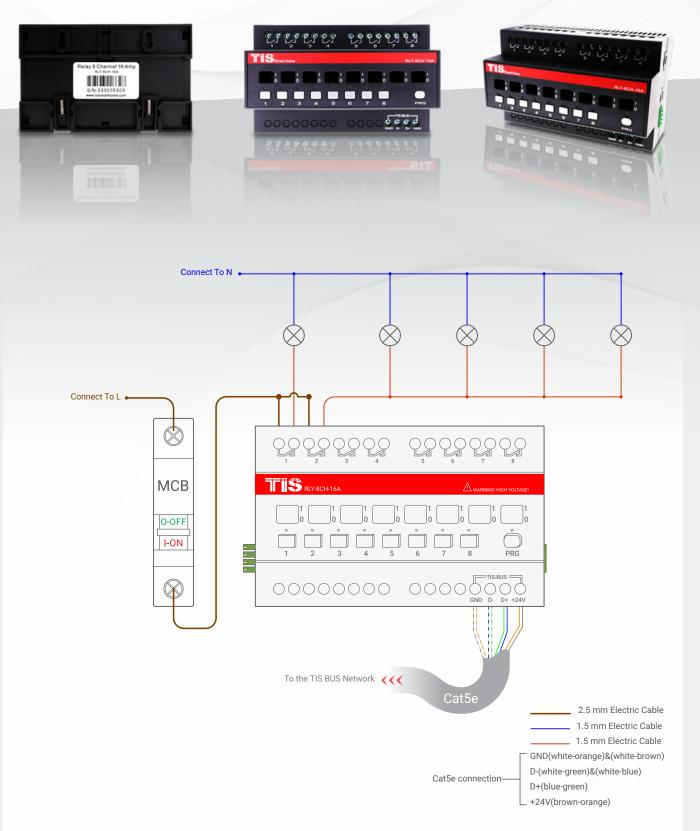
Figure 1: Lights Connection Diagram
