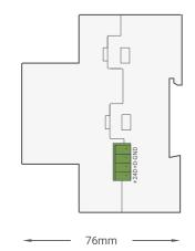
Figure 6: Module's Dimension Diagram
