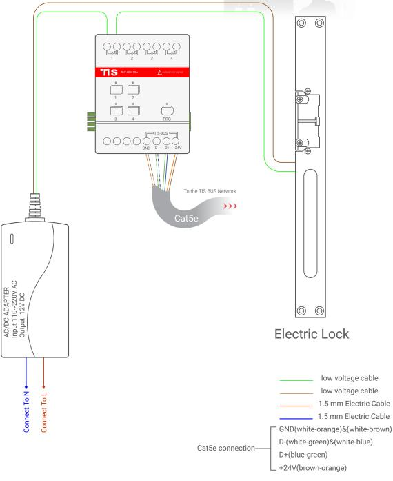
Figure 3: Electric Lock Connection Diagram
