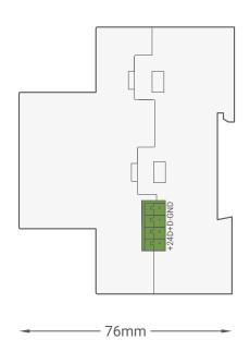
Figure 6: Module's Dimension Diagram
