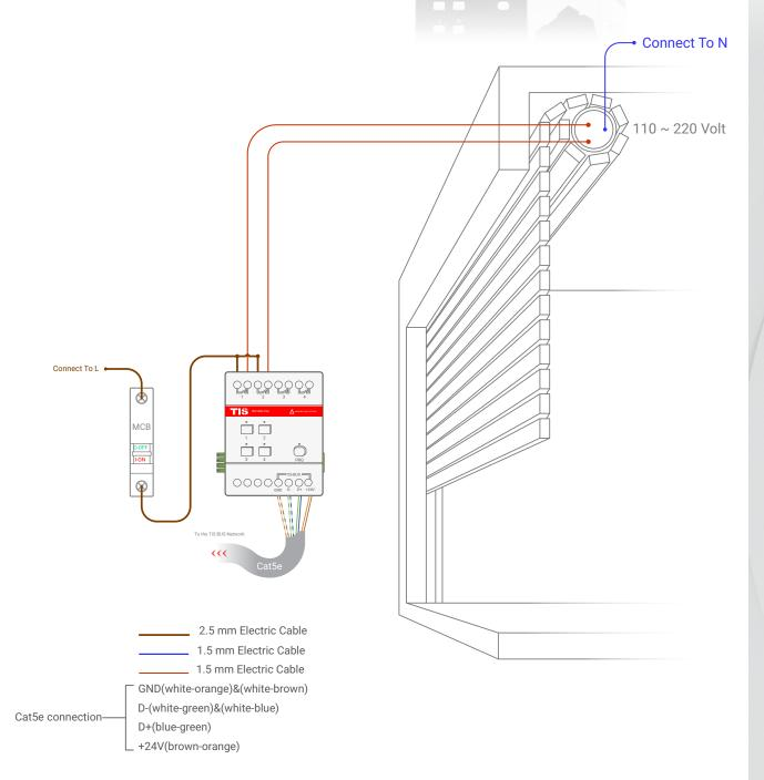
**Figure 2: Motors Connection Diagram**
