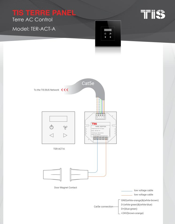
Figure 5: TER-ACT-A & ADD-3DL-12V Magnetic Door Contact Connection Diagram
