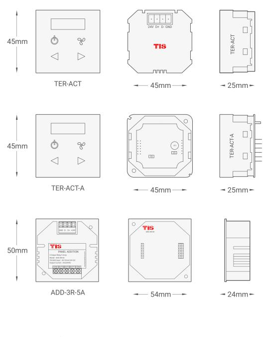
Figure 8: Module's Dimension Diagram
