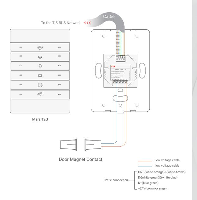
Figure 5: Mars 12G & ADD-3DL-12V Magnetic Door Contact Connection Diagram
