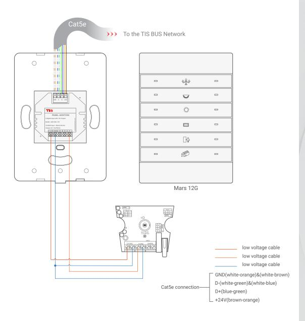
Figure 6: Mars 12G & ADD-3DL-12V 3rd Party Sensor Connection Diagram
