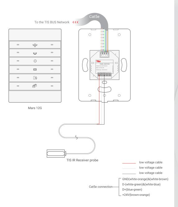
Figure 7: Mars 12G & ADD-2DL-IRR Connection Diagram
