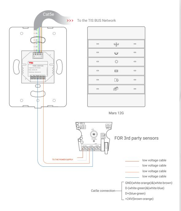
▲ Figure 12: Mars 12G & ADD-2DL-IRE 3<sup>rd</sup> Party Sensor Connection Diagram
