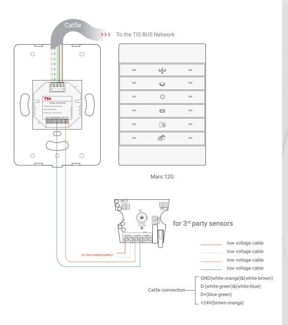
Figure 9: Mars 12G & ADD-2DL-IRR 3rd Party Sensor Connection Diagram
