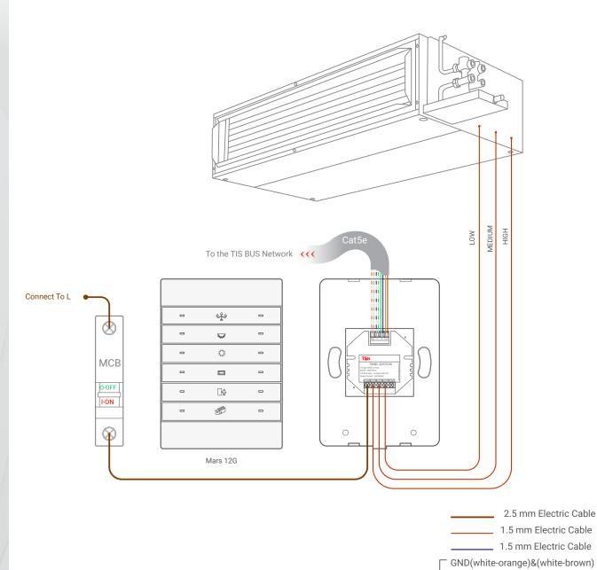
Figure 2: Mars 12G & ADD-3R-5A FCU Connection Diagram
