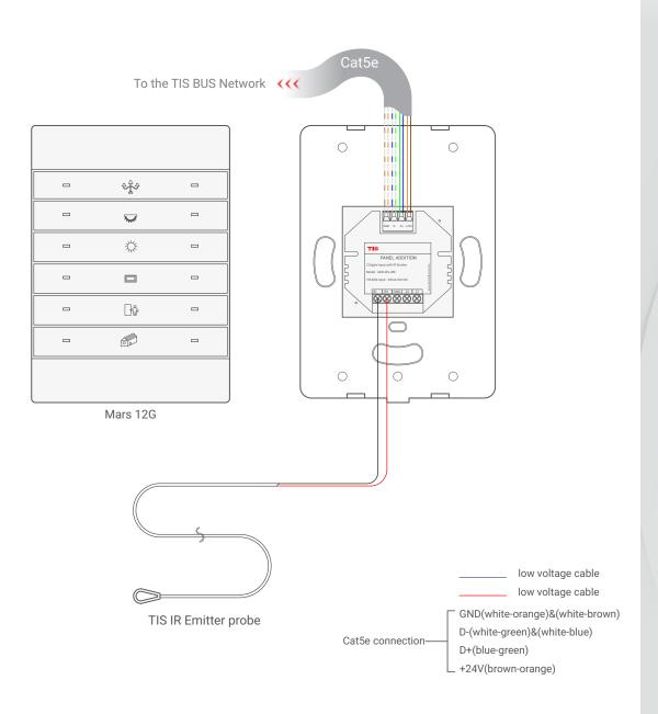
Figure 10: Mars 12G & ADD-2DL-IRE Connection Diagram
