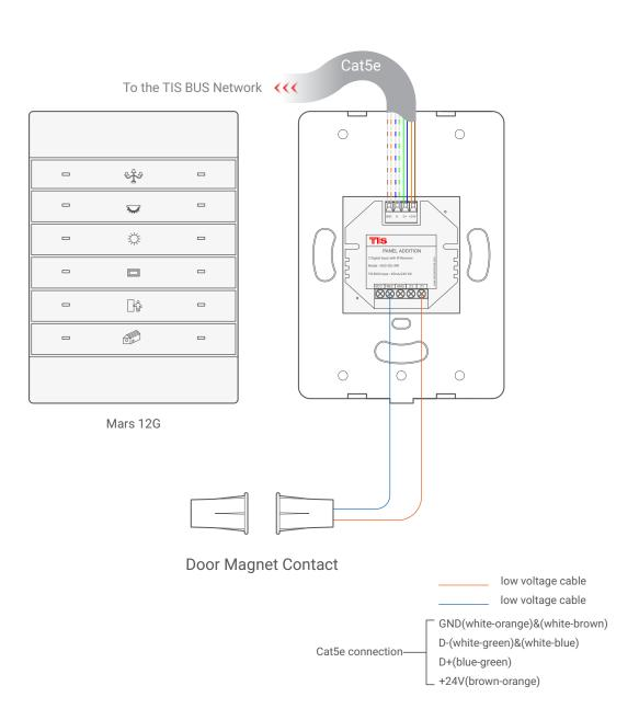
Figure 8: Mars 12G & ADD-2DL-IRR Magnetic Door Contact Connection Diagram
