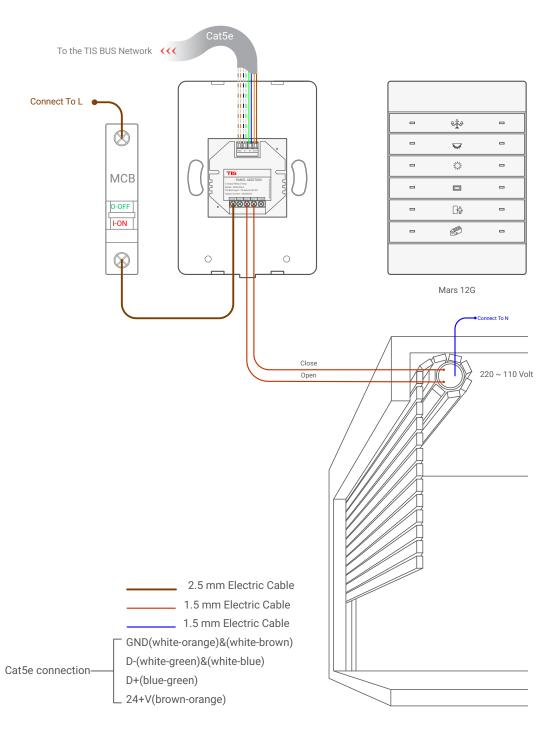
Figure 3: Mars 12G & ADD-3R-5A Motors Connection Diagram
