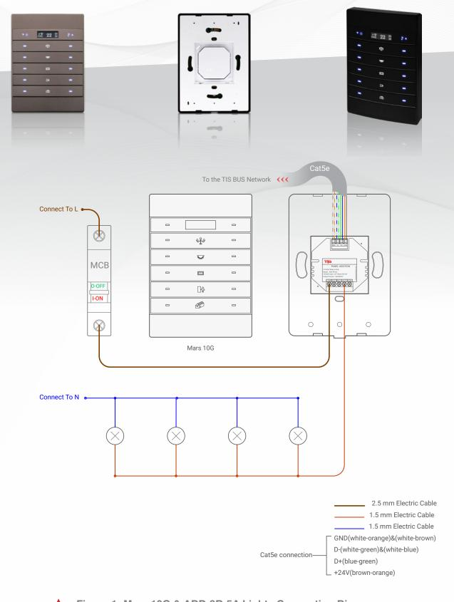
Figure 1: Mars 10G & ADD-3R-5A Lights Connection Diagram
