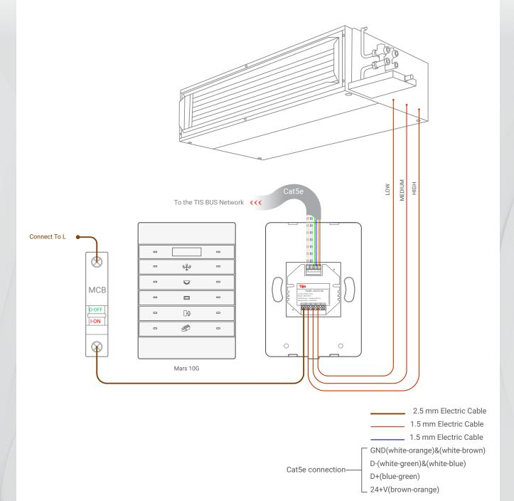
Figure 2: Mars 10G & ADD-3R-5A FCU Connection Diagram
