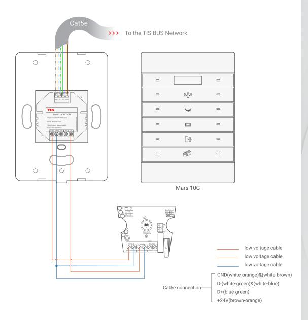
Figure 6: Mars 10G & ADD-3DL-12V 3rd Party Sensor Connection Diagram
