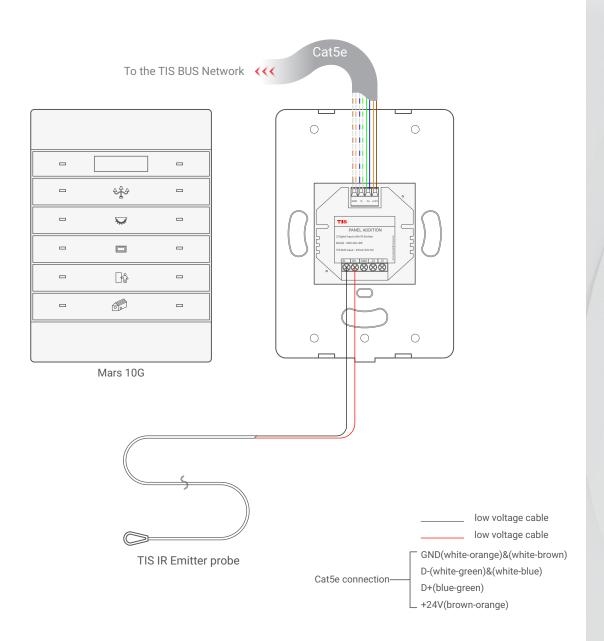
Figure 10: Mars 10G & ADD-2DL-IRE Connection Diagram
