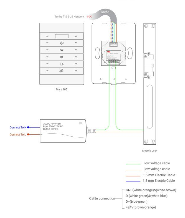
Figure 4: Mars 10G & ADD-3R-5A Electric Lock Connection Diagram
