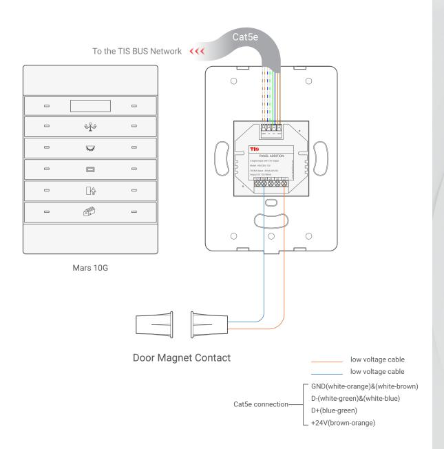
Figure 5: Mars 10G & ADD-3DL-12V Magnetic Door Contact Connection Diagram
