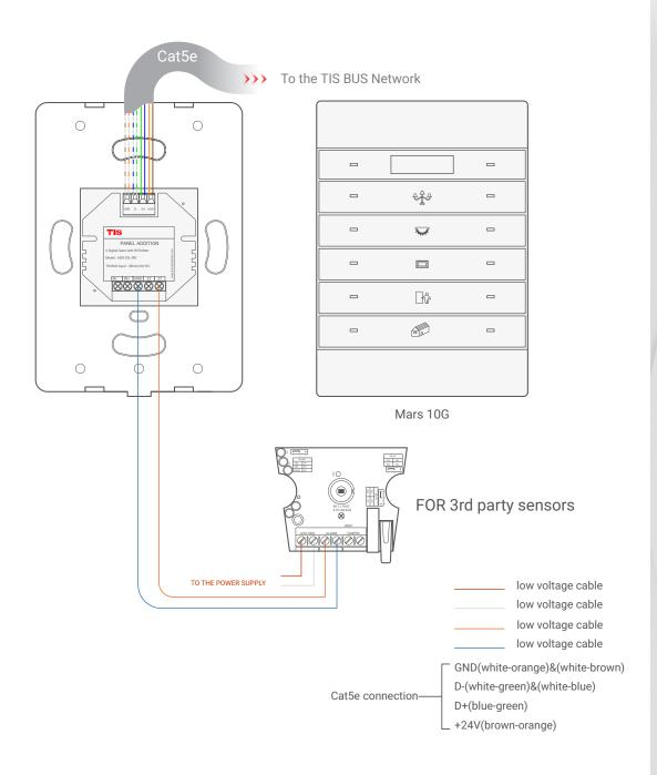
▲ Figure 12: Mars 10G & ADD-2DL-IRE 3<sup>rd</sup> Party Sensor Connection Diagram
