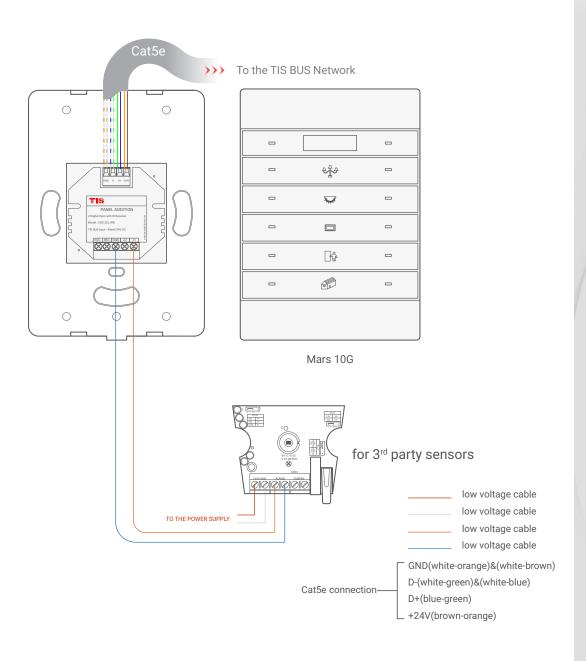
▲ Figure 9: Mars 10G & ADD-2DL-IRR 3<sup>rd</sup> Party Sensor Connection Diagram
