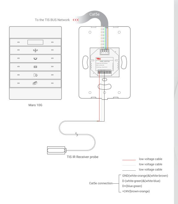
Figure 7: Mars 10G & ADD-2DL-IRR Connection Diagram
