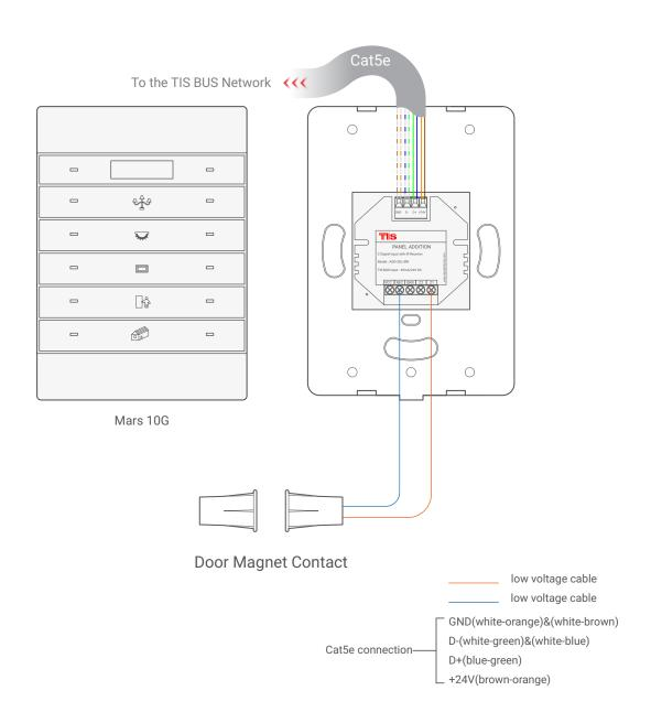
Figure 8: Mars 10G & ADD-2DL-IRR Magnetic Door Contact Connection Diagram
