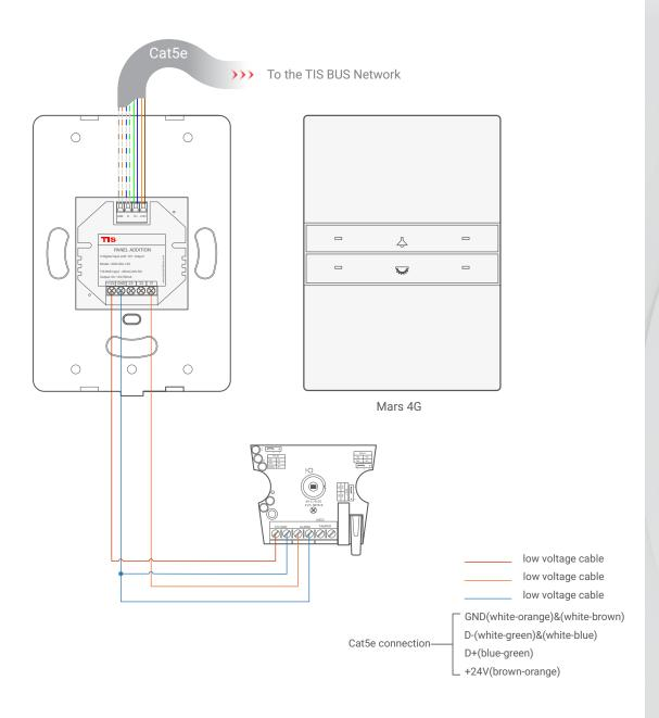
Figure 6: Mars 4G & ADD-3DL-12V 3rd Party Sensor Connection Diagram
