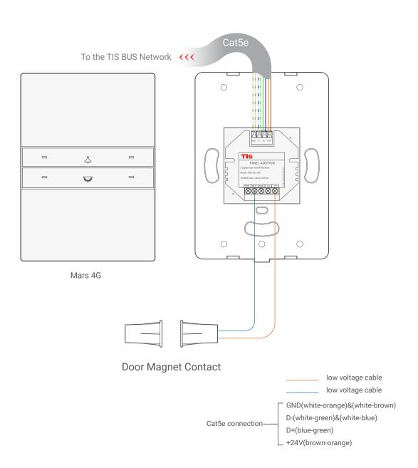
Figure 8: Mars 4G & ADD-2DL-IRR Magnetic Door Contact Connection Diagram
