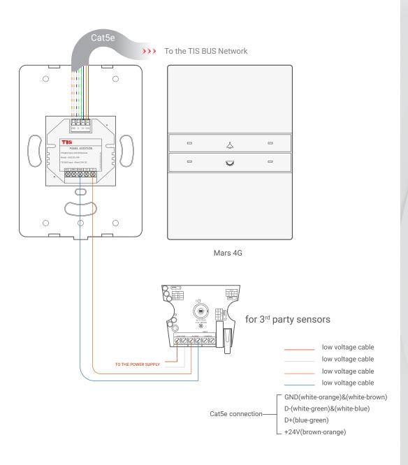
Figure 9: Mars 4G & ADD-2DL-IRR 3rd Party Sensor Connection Diagram
