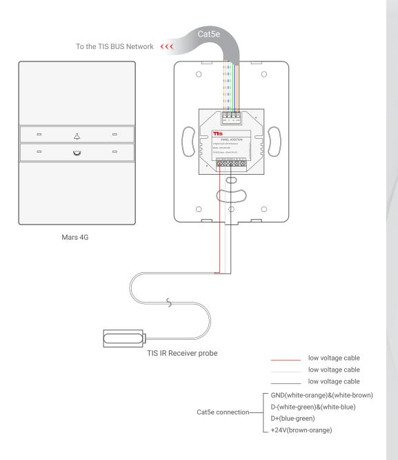
Figure 7: Mars 4G & ADD-2DL-IRR Connection Diagram
