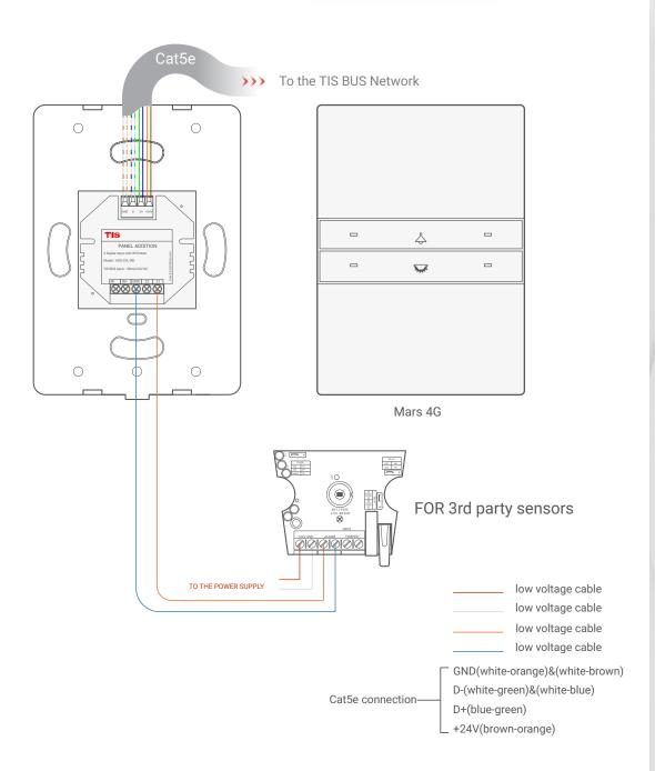
Figure 12: Mars 4G & ADD-2DL-IRE 3rd Party Sensor Connection Diagram
