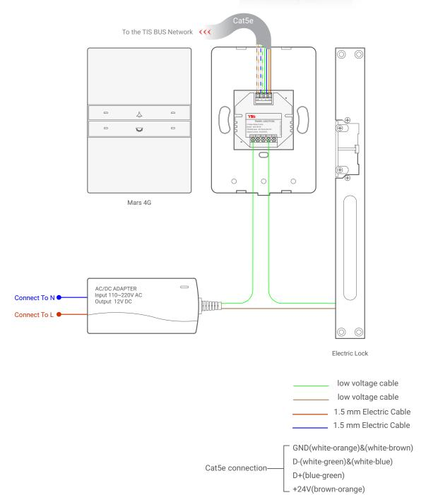
Figure 4: Mars 4G & ADD-3R-5A Electric Lock Connection Diagram
