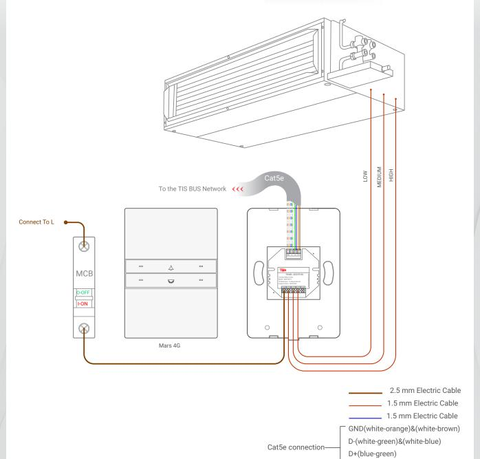
Figure 2: Mars 4G & ADD-3R-5A FCU Connection Diagram
