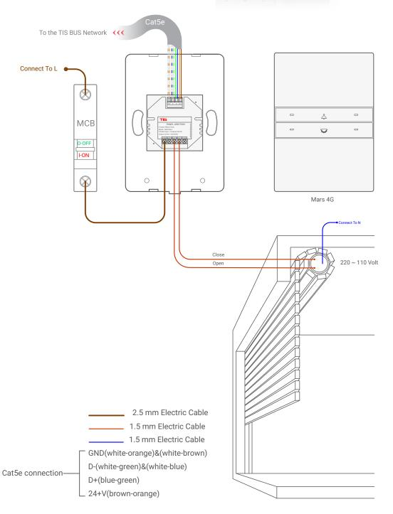
Figure 3: Mars 4G & ADD-3R-5A Motors Connection Diagram
