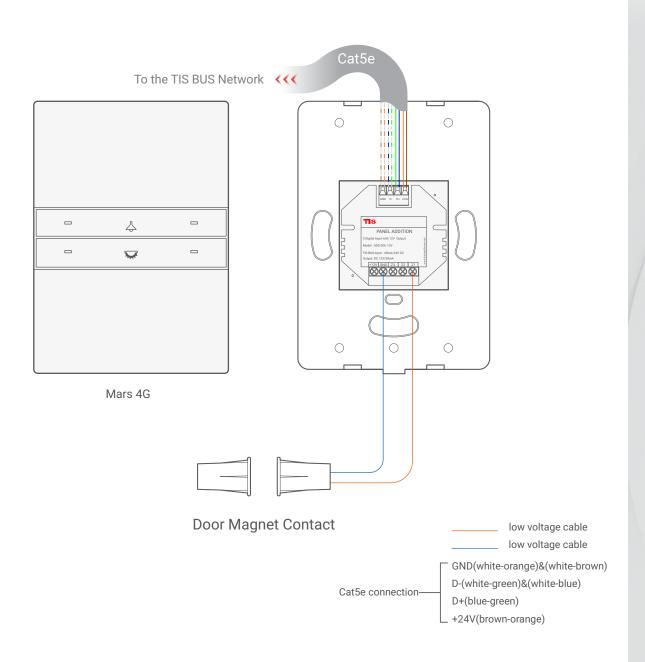
▲ Figure 5: Mars 4G & ADD-3DL-12V Magnetic Door Contact Connection Diagram
