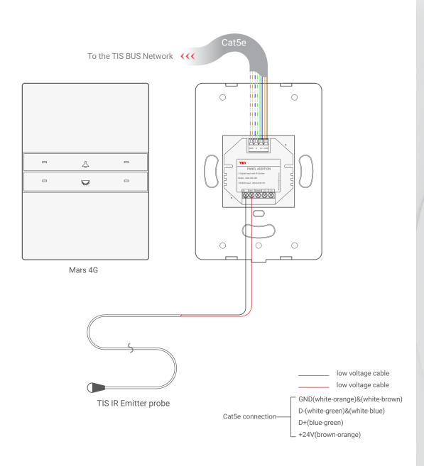
Figure 10: Mars 4G & ADD-2DL-IRE Connection Diagram
