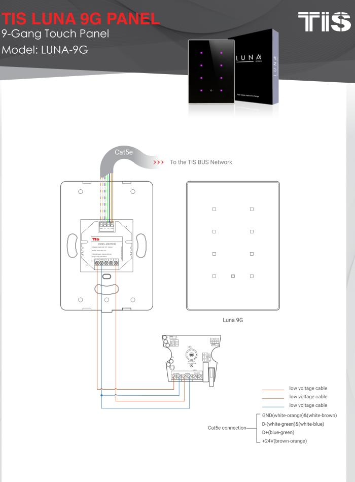
Figure 6: Luna 9G & ADD-3DL-12V 3rd Party Sensor Connection Diagram
