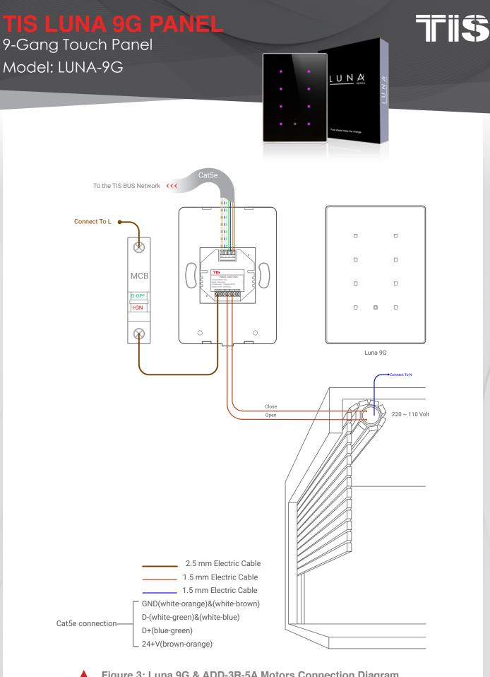
Figure 3: Luna 9G & ADD-3R-5A Motors Connection Diagram
