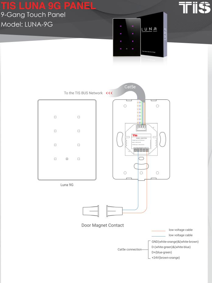
Figure 8: Luna 9G & ADD-2DL-IRR Magnetic Door Contact Connection Diagram
