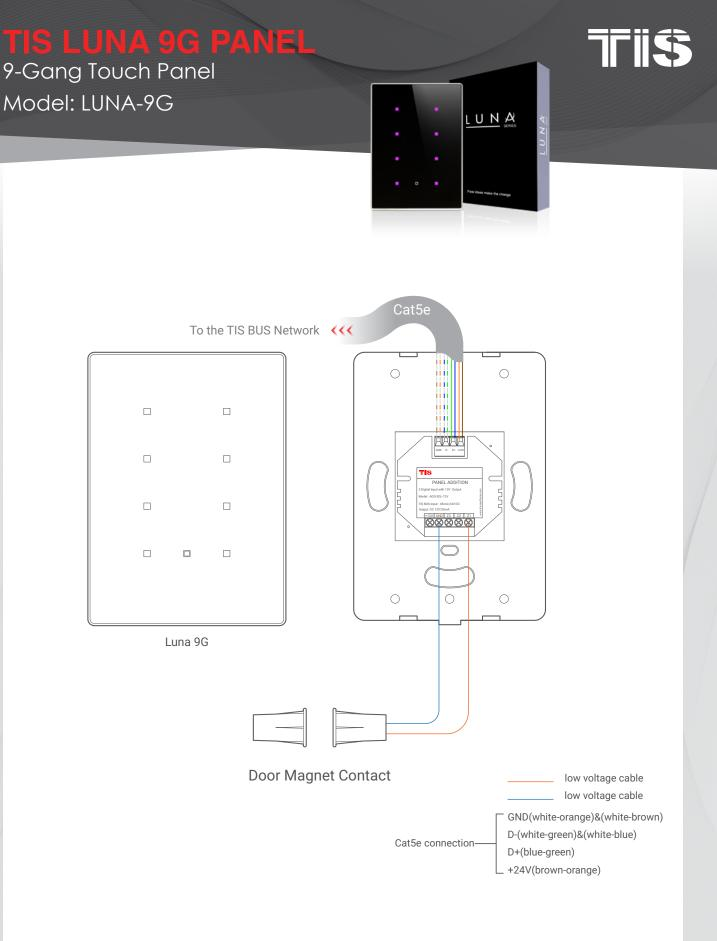
Figure 5: Luna 9G & ADD-3DL-12V Magnetic Door Contact Connection Diagram
