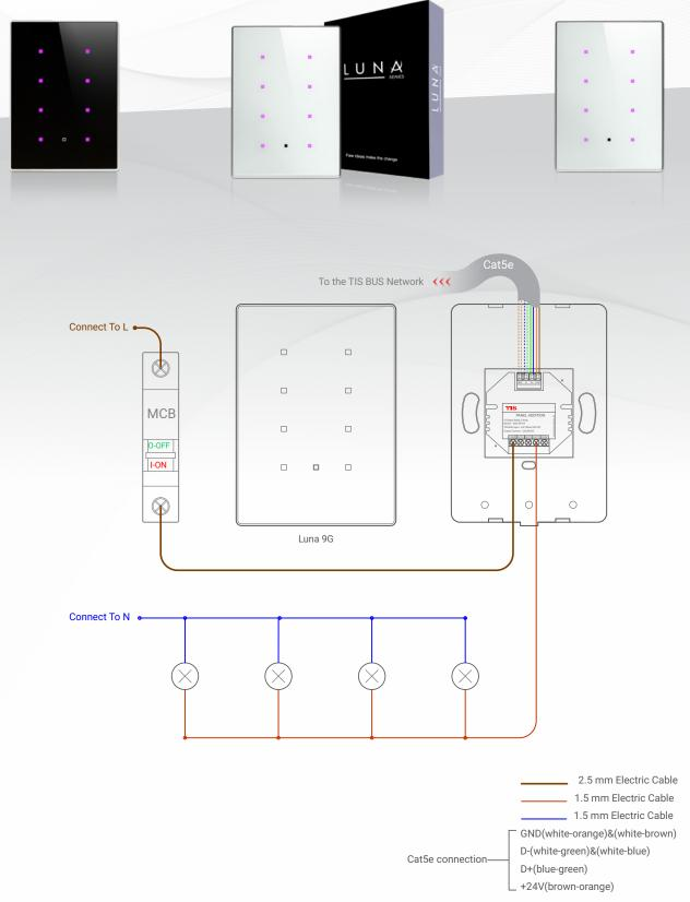
Figure 1: Luna 9G & ADD-3R-5A Lights Connection Diagram
