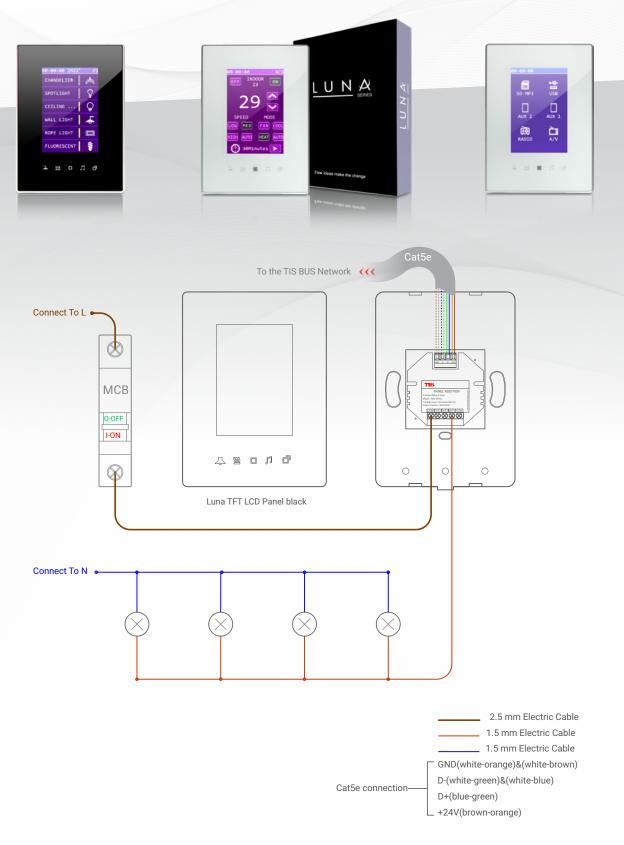
Figure 1: Luna TFT & ADD-3R-5A Lights Connection Diagram
