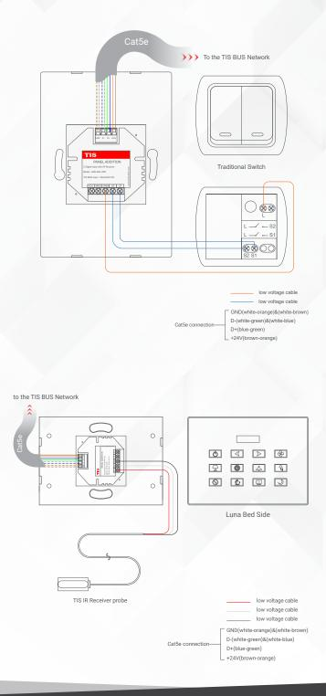
You can add an External Infrared Receiver to the IRR Port, connect as follows:
