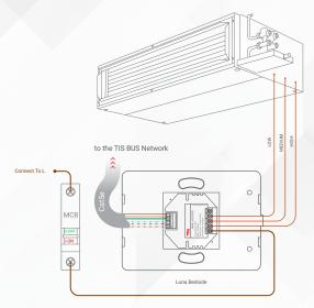
2.5 mm Electric Cable 1.5 mm Electric Cable 1.5 mm Electric Cable GND(white-orange)&(white-brown) D-(white-green)&(white-blue) D+(blue-green) 24+V(brown-orange)
