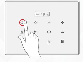
3>> Test your air conditioning by changing the mood, Heat/Cool, and fan speed from low to medium to high. HVAC module should respond accordingly.
