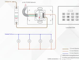
2.5 mm Electric Cable 1.5 mm Electric Cable 1.5 mm Electric Cable GND(white-orange)&(white-brown) D-(white-green)&(white-blue) D+(blue-green) +24V(brown-orange)
