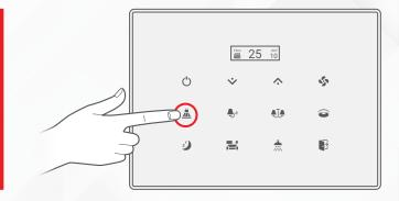
Long press any button from 5-8 for 12 seconds until its LED blinks RED.
