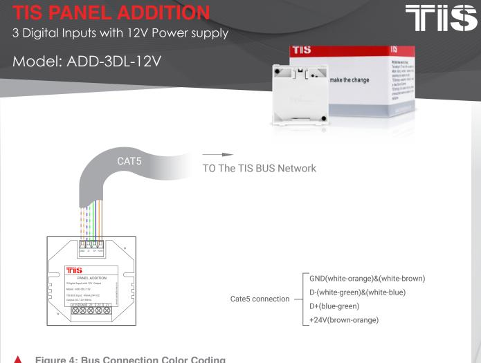
Figure 4: Bus Connection Color Coding
