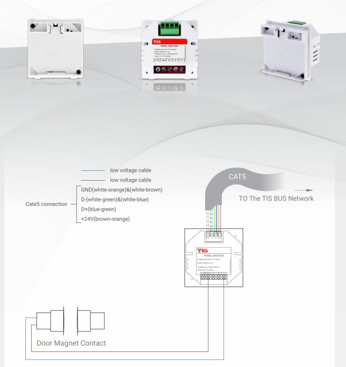
Figure 1: Magnetic Door Contact Connection Diagram
