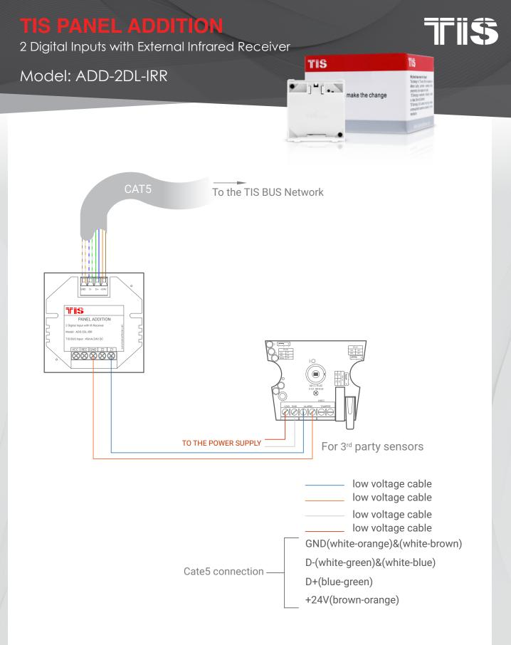
Figure 2: ADD-2DL-IRR & 3<sup>rd</sup> Party Sensor Connection Diagram
