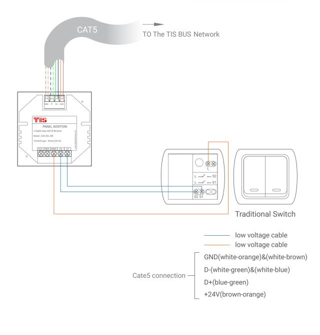
Figure 4: Traditional Switch Connection Diagram
