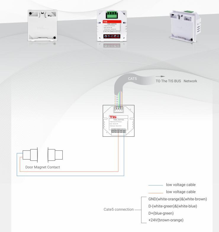
Figure 1: ADD-2DL-IRR & Magnetic Door Contact Connection Diagram
