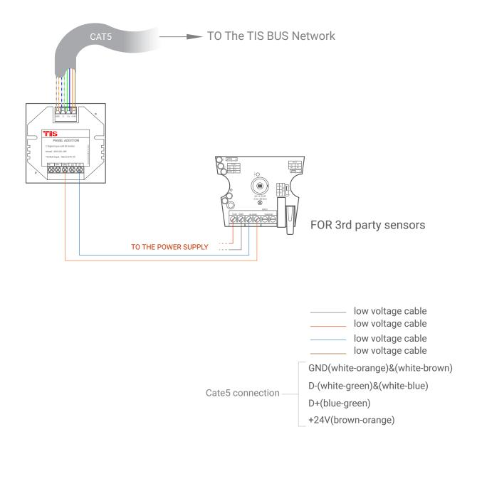
Figure 2: ADD-2DL-IRE & 3<sup>rd</sup> Party Sensor Connection Diagram
