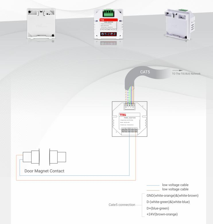
Figure 1: ADD-2DL-IRE & Magnetic Door Contact Connection Diagram
