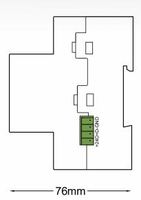
Figure 1: Module Dimensions
