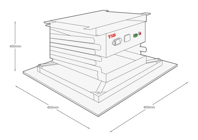
Figure 3: Module's Dimensions
