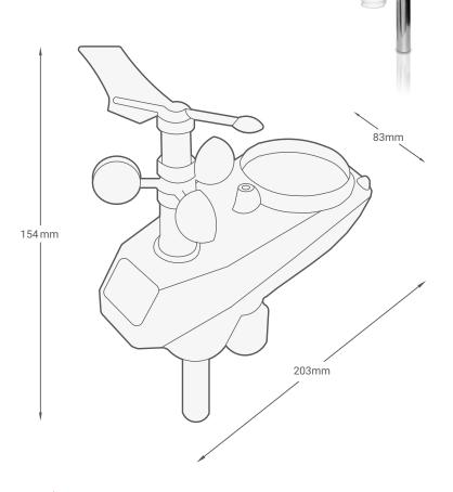
Figure 3: TIS-WS-71 Module's Dimensions
