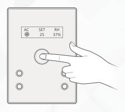
Test your air conditioning by changing the 3 fan speed from low to medium to high. Your relay should respond accordingly.
