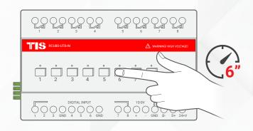
On the IO Push buttons, shortly press on **2** any push button or press the wall switch that is connected to the dry inputs of the panel addition zones.
