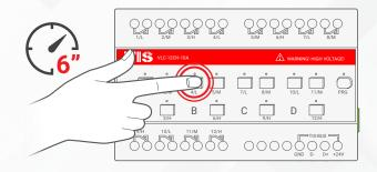
**2** On the IO AC page, push the IO knob to turn the AC ON.
