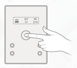
Test your floor heating by changing the 3 **>>** temperature; the relay should respond accordingly.
