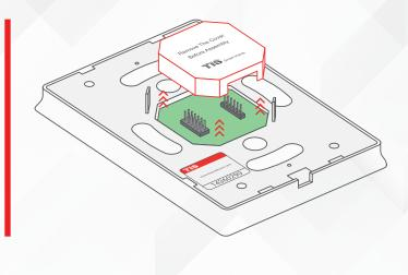
**10** Connect the main Luna panel vertically to the part installed on the wall; install the upper part by making sure the buckles are completely inside.
