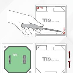
Connect the Wall Base and Panel Addi-**4** tion in this position. Place the upper pins as shown, and then push the down pins down with your fingers to assemble.
