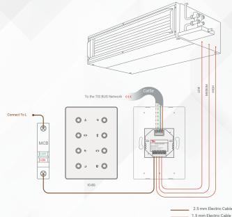
2.5 mm Electric Cable 1.5 mm Electric Cable 1.5 mm Electric Cable 1.5 mm Electric Cable (white-orange)&(white-brown) D-(white-green)&(white-blue) D+(blue-green) 24+V(brown-orange)
