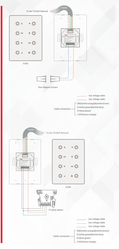
Also, you can connect any 12V operated smoke detector or any 3<sup>rd</sup> party sensor with NC/NO connection to the 12V GND and Z1-Z3 terminals as per the diagram.
