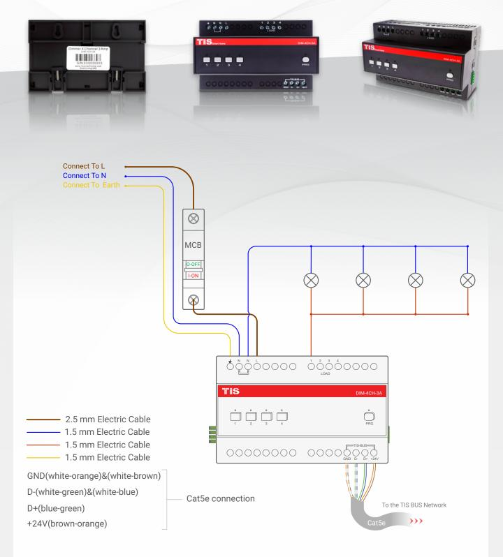
Figure 1: Lights Connection Diagram
