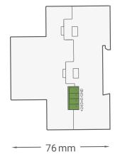
**Figure 4: Module Dimensions**
