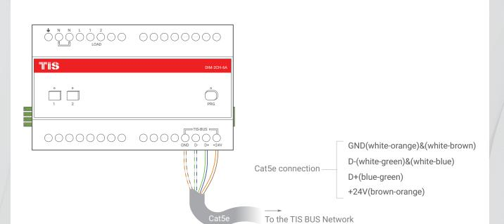
Figure 2: BUS Connection Color Coding
